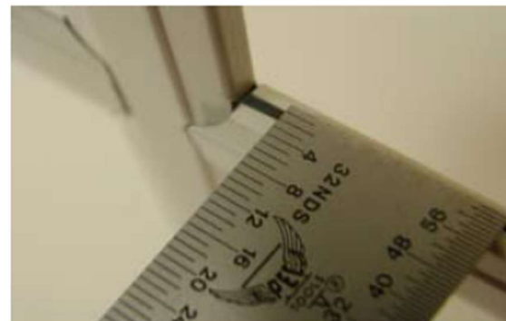
Unacceptable – Greater than 1/32" Figure 5
